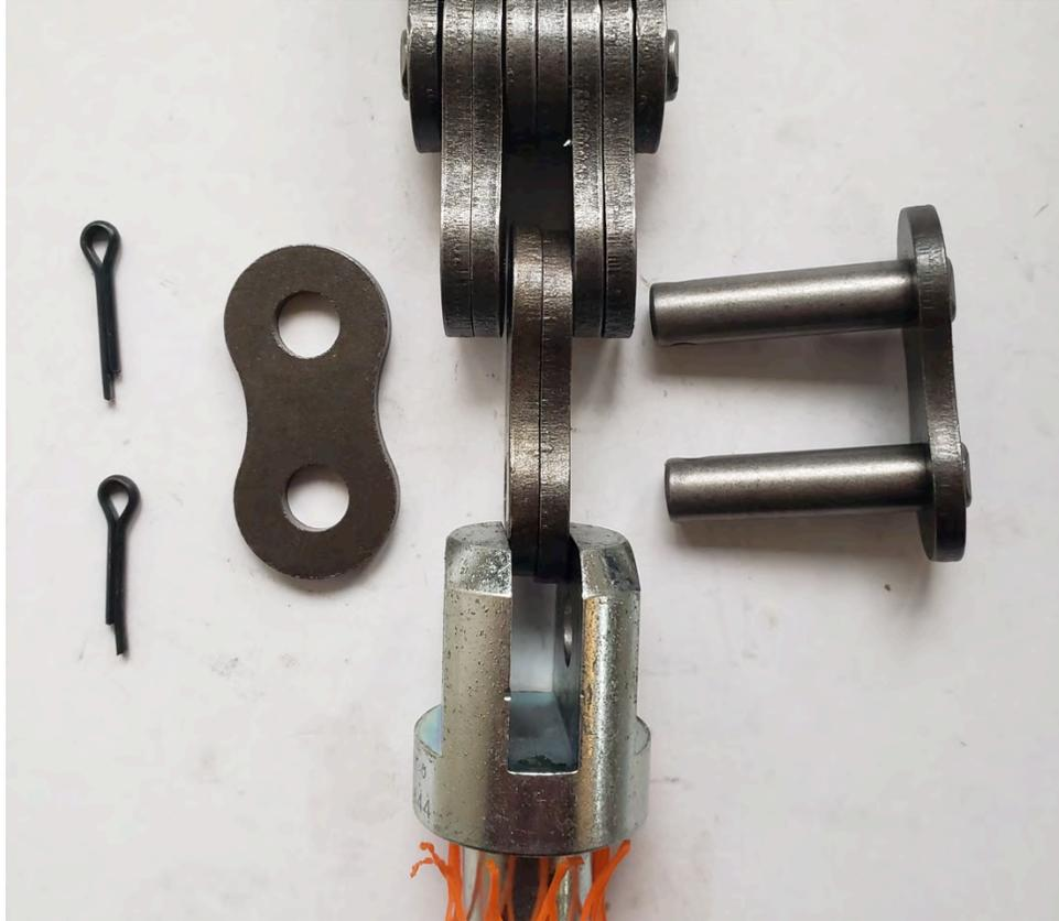
Align the plates before assembling. Then insert the Connecting link through both the chain and the Type B LCA.
