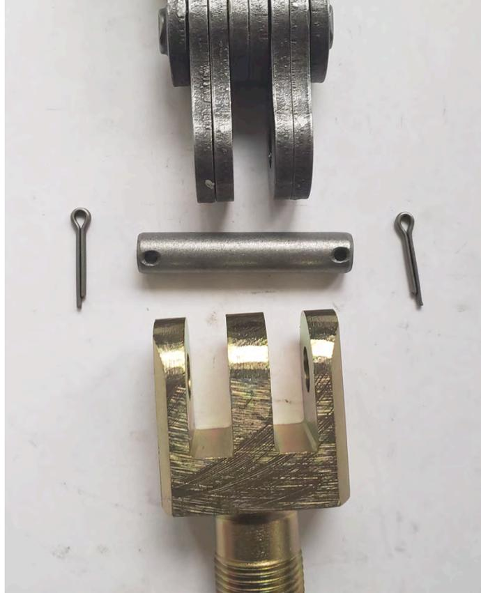
Insert the Male end of the chain into the Type A LCA and slide the Clevis pin through the holes. Secure with a split pin on either side.
