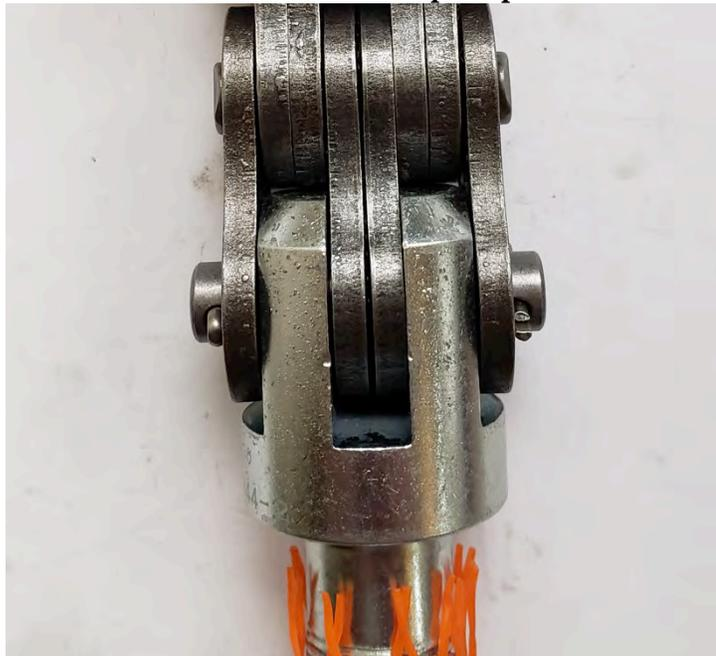
The final step in securing either the Connecting Link or Clevis Pin is to bend the split pin. The split pin does not take direct load and only needs to be bent enough to prevent it from falling out of the holes in the Connecting Link or Clevis Pin.
