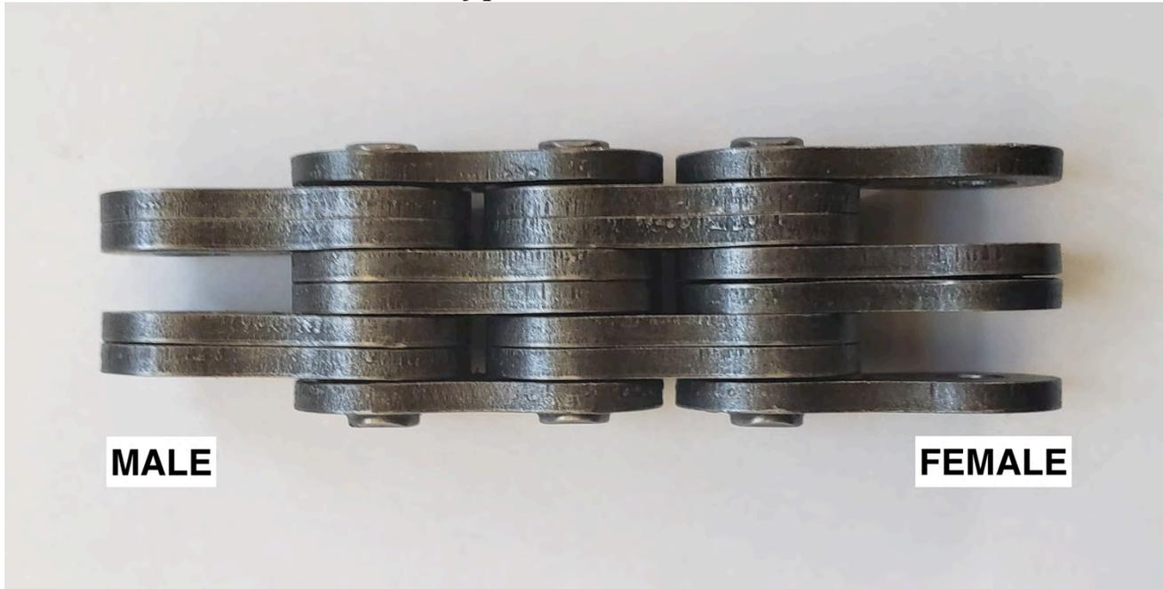
Depending on which pin is removed to separate the chain, the resulting end will be either Male or Female.
