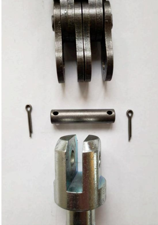
Align the Female chain end with the Type B LCA and insert the Clevis Pin through the holes in both the Female chain end and the Type B LCA (A hammer or reamer are often required to get the pin through the exterior plates). Secure the Clevis Pin with split pins on either side.
